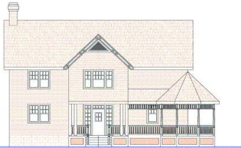
Incorporate details such as double hung windows, gables, decorative trim, turrets and porches.
