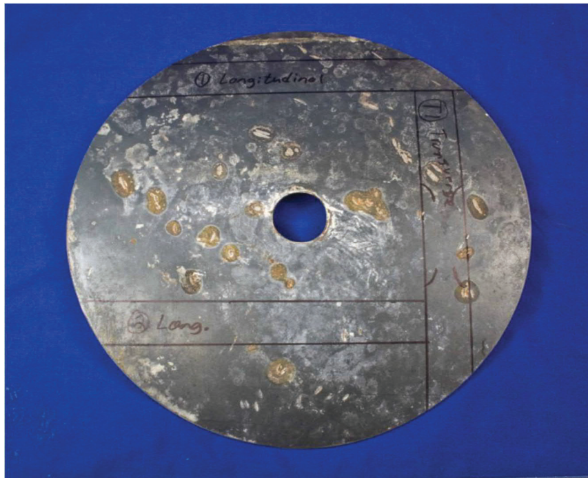
Figure 3: Tensile Specimen Locations in Steel Cylinder (note weld along top of coupon)
