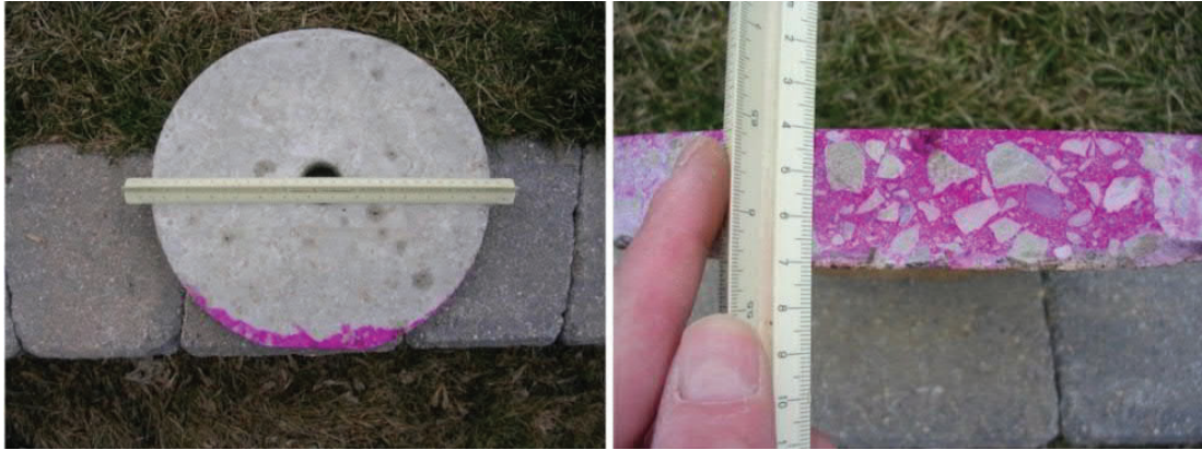
Figure 4: Cement Degradation (pH) Test of Concrete Pipe Core.
